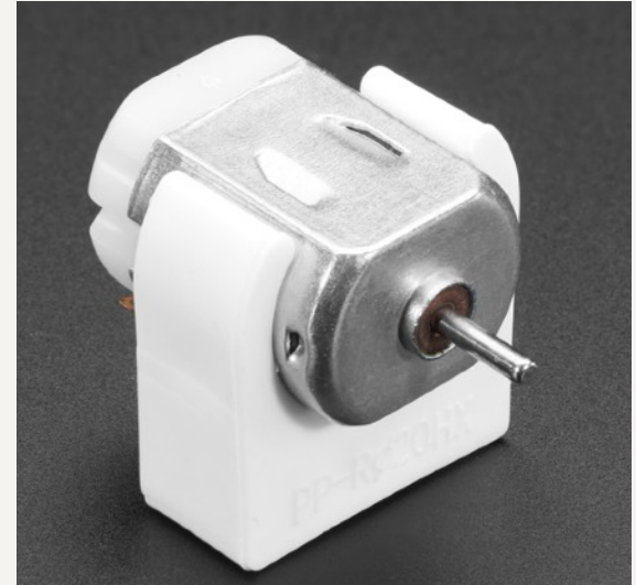
Common toy & small electronics motor called “130”
